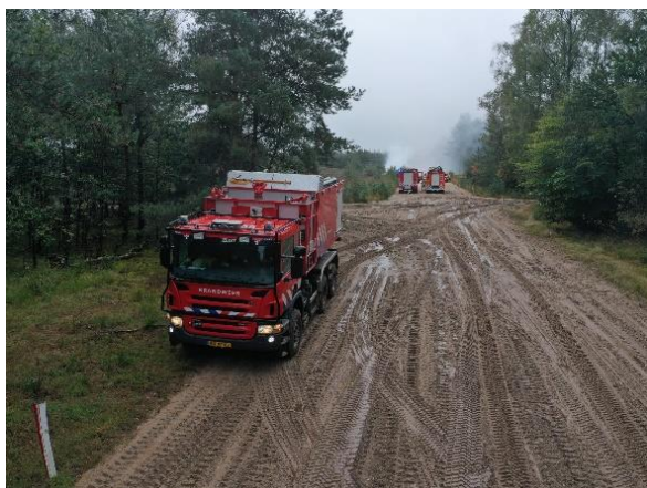
Figure 59. Use of an all-terrain water truck to provide extra water for the engines that are extinguishing a wildfire.
