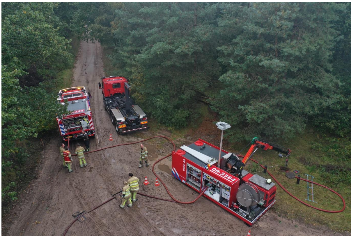
Figure 58. Use of a high-capacity pump to pump up water from more than 50 metres below the surface.
