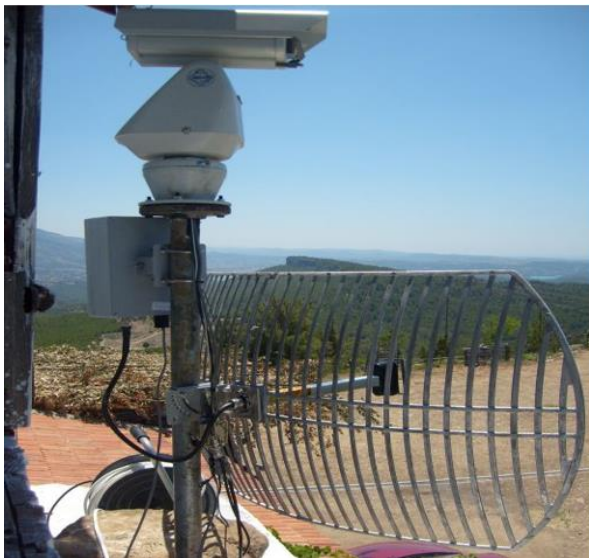
Figure 113. The early warning system for detecting forest fires and automatic fire-finding systems established and put into service via a joint project among GDF, Bilkent University and Scientific and Technological Research Council of Türkiye(TÜBİTAK) for a decade.
