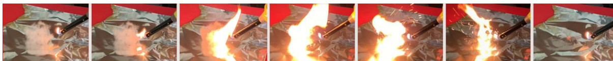
Figure 106. Images from a video when testing fire behaviour of aspen fluff in the laboratory. The fluff burned extremely fast. Residence time about 0.3 second. Photo: Anders Granström, SLU
