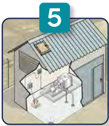
Borehole with a motorized pump
