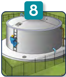
Piped distribution: storage tank
