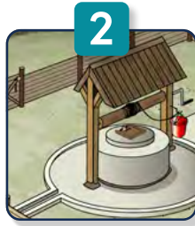
Dug well with a windlass
