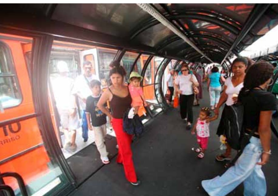
Low floor BRT eases access in Curitiba, Brazil. (Photo: Ron Gilling/Brazilie Lineair/Still Pictures)
